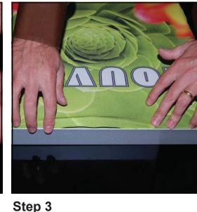
Once all corners are inserted, press one silicon edge into channel from corners and work toward the center.
